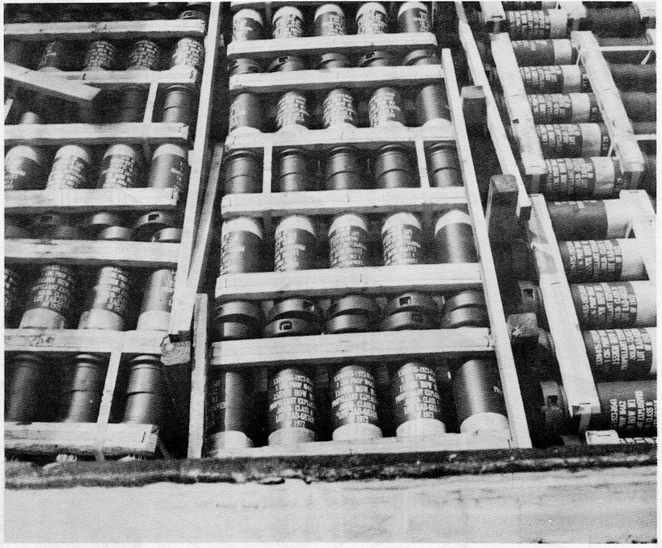
Figure 9-25. Stowing and securing of M4A2 propellant charges in tween-deck compartment.
