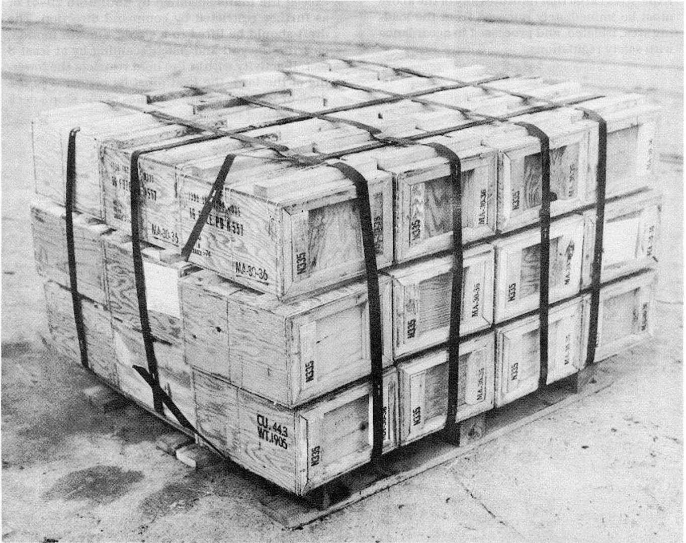
Figure 42. Unit load isolated because of defective banding.
