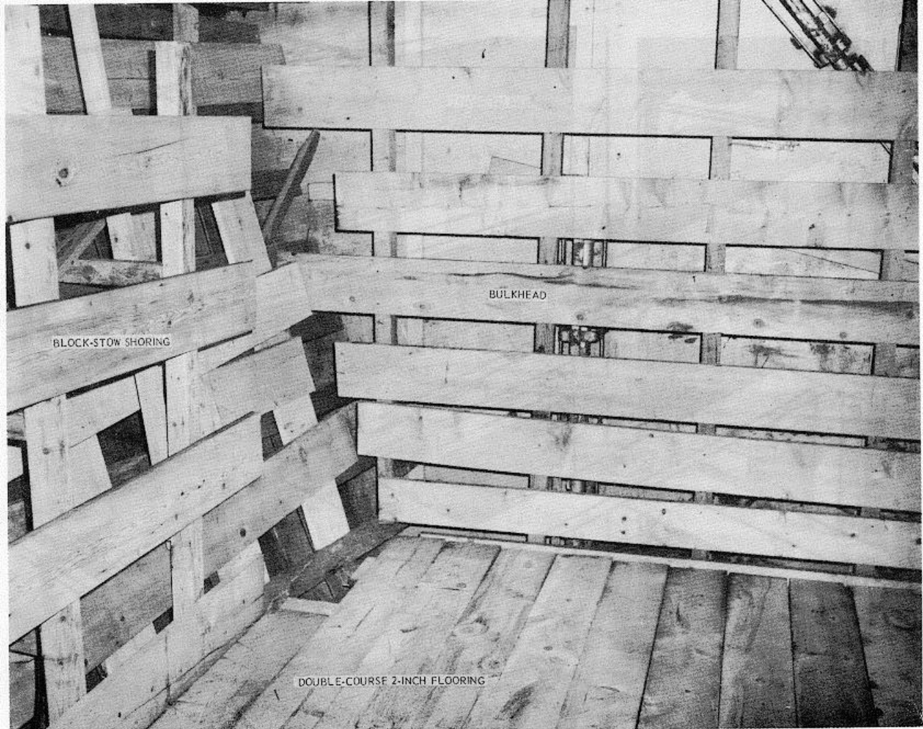
Figure 9-44. Typical preconstructed shoring for block stowage of 500-pound bombs in lower holds.
